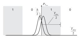
Fig. 6. Offset compensated mod 2 quantization.
