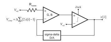
Fig. 2. Amplification-based RBG.
