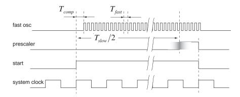
Fig. 8. Waveforms of the main signals.
