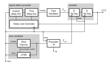
Fig. 7. Detailed block scheme for the proposed RBG.
