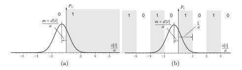
**Fig. 1.** Source quantization modes: (a) sign-mode (x[i] = sign(s)), (b) mod 2-mode  $(x[i] = \lfloor s \rfloor \mod 2)$ .
