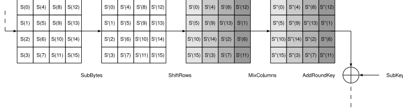
Fig. 1. SubBytes, ShiftRows and MixColumns operations [15]
