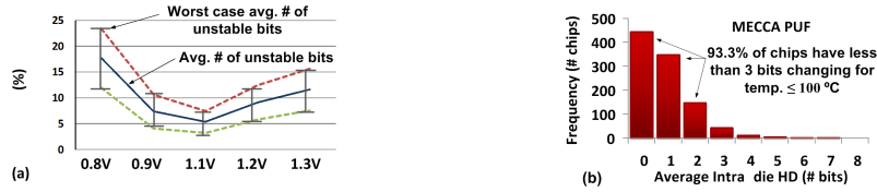
Fig. 8. Average intra-die HD from 1000 chips for MECCA PUF (a) for supply voltage variation (compared to nominal V_{dd}=1V ), and (b) for temperature variation.
